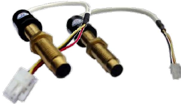
1. Function: 3NSS102K is a device that measures velocity, which works face is induced by moving of ferric metallic object, so it can measure the velocity of gears, rack etc. It is frequency used in some occasions where want to measure rotary speed, for example speed vary feeders (3N-PT, 3N-TJL).
